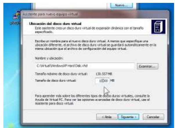
(6) Assign to the virtual harddisk sufficient memory, at least 10000 MB = 10 GB
